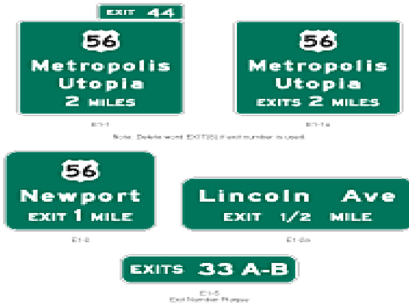
Figure 8E-16. Examples of Interchange Advance Guide Signs
